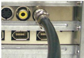
Connecting TV antenna to the tuner card
